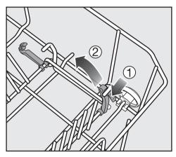
Press the yellow lever down ① and fold the spikes down ②.
